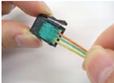
Inset the wire to be connected
